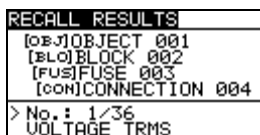
Figure 7.1: Data structure and measurement fields
