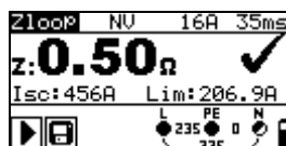
Figure 5.25: Example of loop impedance measurement result
