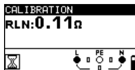
Figure 5.14: Results with old calibration values
