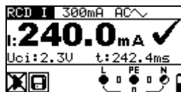
Figure 5.20: Trip-out current measurement result example
